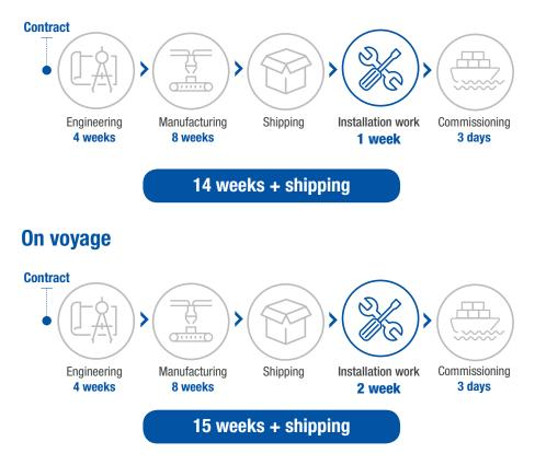
BWTS retrofit takes an average of 13 weeks and a separate period for product delivery is needed to complete the installation after the contract.
