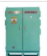
The major function of Power Supply Panel is to operate the medium pressure UV lamps UV. It controls the strength of UV lamps with the capacitors mounted in the Panel. Also it detects whether the UV lamps are functioning properly or not. The temperature sensor is mounted inside to monitor temperature in order to give an alarm to an operator and shut down the system in case of overheating.
