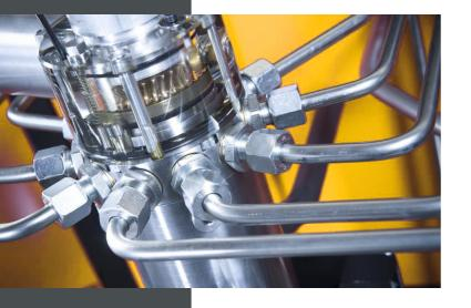
Our company is an agent manufacturer of an innovative cylinder lubrication system for two-stroke diesel engines. The patented Hans Jensen Cylinder Lubrication System can reduce cylinder oil consumption by up to two times and reduce sleeve wear by several times.
