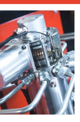
The complete system consists of a number of HJ Lubtronic lubricators, 1 per cylinder, each connected to a local controller – in an arrangement.
